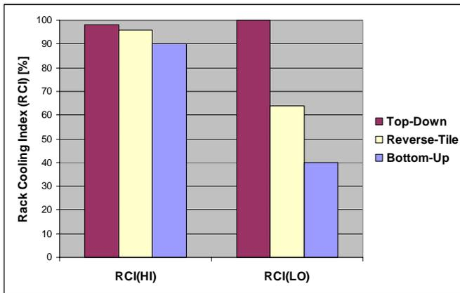
Figure 7. RCI Comparison of the Three Systems at  $150 \text{ W/ft}^2$  ( $1,615 \text{ W/m}^2$ )
