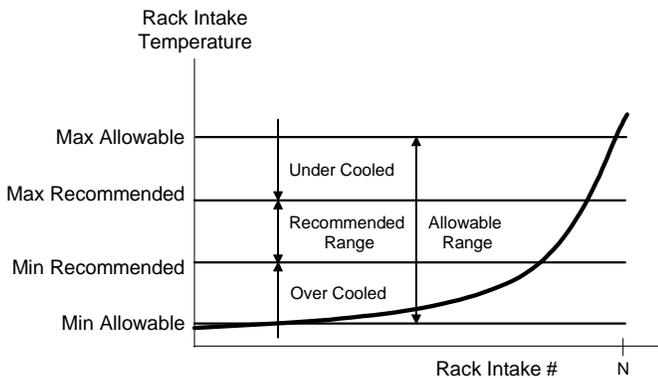
Figure 6. Temperature Distribution (hypothetical), Thermal Ranges, and Thermal Limits
